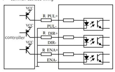
Notice: when control signal voltage VCC = 24V,
